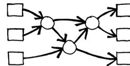
3. Below are two different networks that will sort four inputs. Which is the faster? (The second one is. Whereas the first requires all comparisons to be done serially, one after the other, the second has some being performed at the same time. The first network is an example of serial processing, whereas the second uses parallel processing to run faster.)
